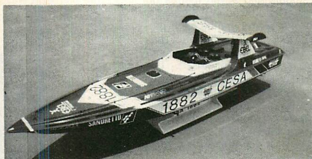
TECHNICAL DATA: WEIGHT 1.8KG, LENGTH 101CM, BEAM 22CM, WINGSPAN 30CM, POWER 2X700 RST 21,000 RPM MOTORS
