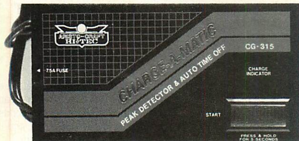
Operation of this charger couldn't be easier. Connect the input to 12v battery, the output to your Ni-Cad pack and hold down the button for 5 seconds. An indicator lamp will glow. When your pack is fully charged the unit will automatically switch off and the lamp will blink. The charged pack should be just warm to the touch.
