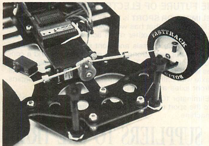
Competition front end is adjustable via five locknuts.
