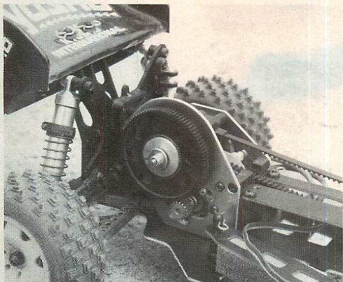
New Lazer features a centre differential behind spur gear.
