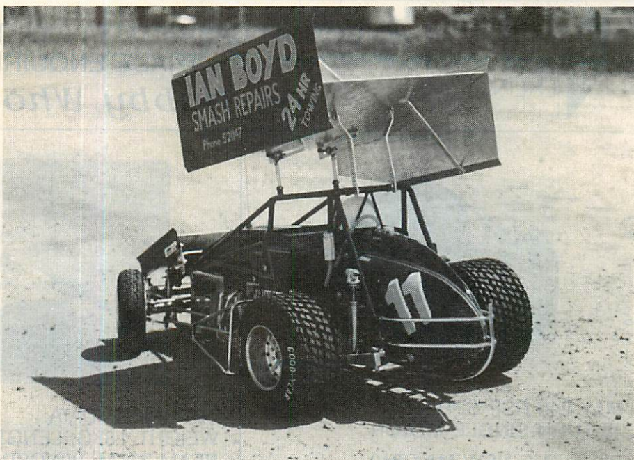
Not your average RC cars. These quarter scale beauties are powered by chainsaw motors of up to 35cc and after using methanol fuel. Most cars have a centrifugal clutch while some opt for direct drive. Steering servo is a beefy Futaba S114 (sail winch) servo in the 14g torque range.
